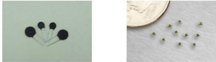
Figure 2.37: Surface contact thermistors.
