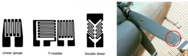
Figure 2.22: Metal-foil strain gauges.
